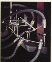
The fixturing available in our indexing turntables machines is extensive and flexible. Often, Empire creates fixtures to handle different parts within the same machine.
