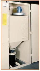
ProFormer cabinets are equipped with cartridgetype dust collectors to facilitate a quick change of filtration surfaces. These two cartridges have a filtration area of 103 square feet each, providing a total of 206 square feet, and can be replaced in minutes through the cabinet door. As a result, loose dust falls into the cabinet rather than onto the work floor.
